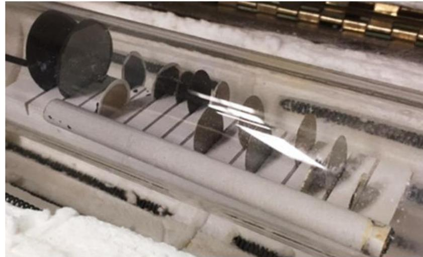
Different solid oxide cells in the reactor for the stability test
