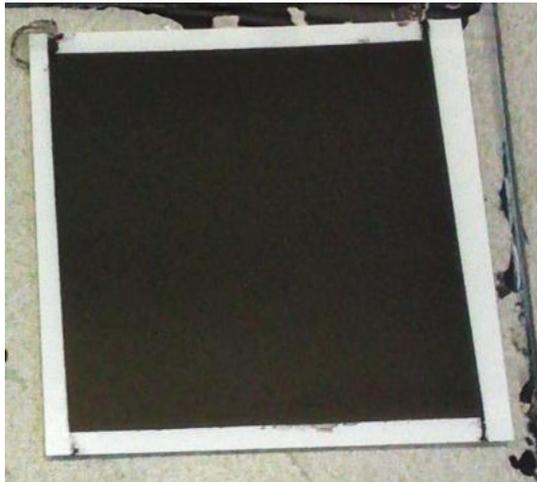
Oxygen electrode on 50 x 50 mm<sup>2</sup> cells
